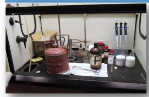
Equipment inside your lab fume hood should be set up to allow for air flow across the face. Some general rules include:
