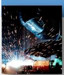
**Shielded Metal Arc Welding (SMAW or Stick)** The coated stick contains the flux which makes this type of welding portable and quick because there is no need for a wire feed system or shielding gas.
